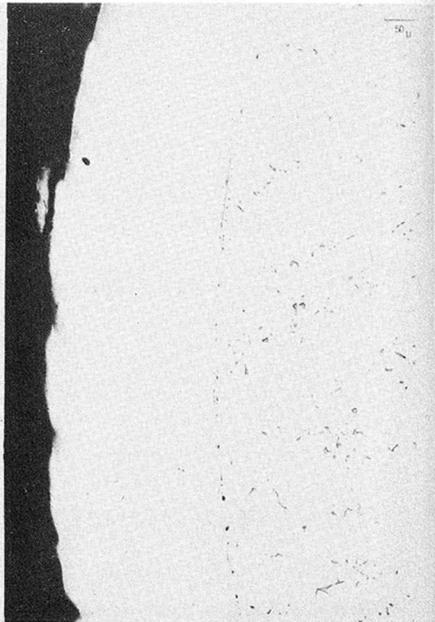
Fig. 12 (b) CoCrAlY cladding on IN-738
